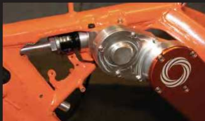
Transfer gearbox requires substantial frame mods
