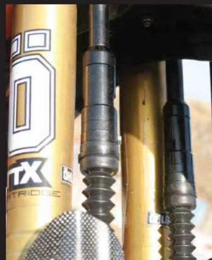
Twin drive shafts to the front hub eliminates torque-steer
